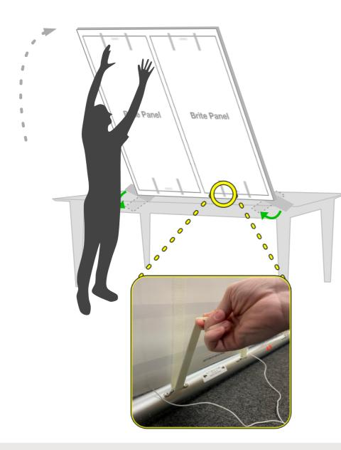
Step 7. Stand the frame up, allowing the lights to stretch as far down as they can.
