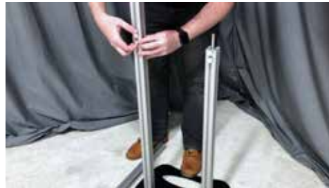
6. Slide thumbscrews to span both extrusions & tighten to secure extrusion legs together.
