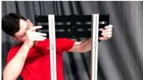
8. Place monitor bracket on top of both extrusion legs.
