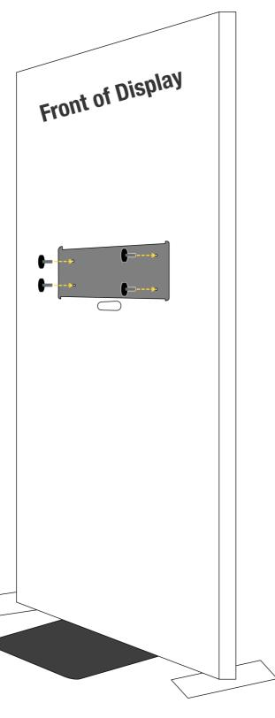
Thumb Screws to attach monitor hanging plate
