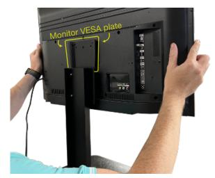
**STEP 4:** Monitor Installation: Be sure your VESA Plate is connected to your monitor. Lower monitor VESA plate onto support arm plate
